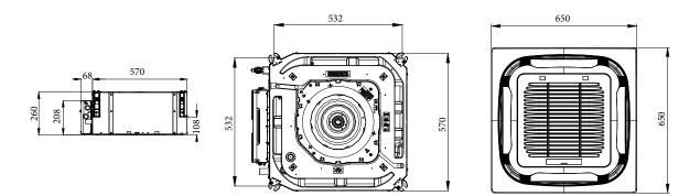
\_\_\_\_\_6.3KW,7.1KW,8.0KW,9.0KW AUX-C-63ARV/I, AUX-C-71ARV/I, AUX-C-80ARV/I, AUX-C-90ARV/I
